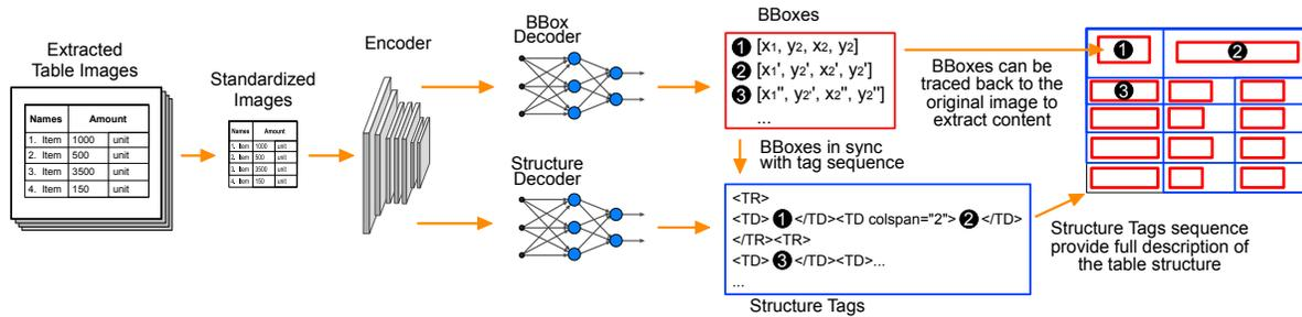
Figure 3: **TableFormer** takes in an image of the PDF and creates bounding box and HTML structure predictions that are synchronized. The bounding boxes grabs the content from the PDF and inserts it in the structure.
